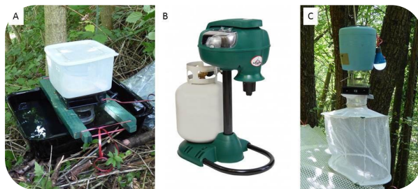
(A) Gravid trap®, (B) Magnet trap® e (C) CDC-trap (Foto: F. Baldacchino; http://www.mosquitomagnet.it/ )
